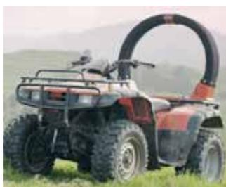
The ATV Lifeguard and Quadbar models referenced in the standard are as at 6 April 2019. However, the standard supports quad bike and aftermarket OPD manufacturers to develop designs for innovative OPDs to protect operators as long as it offers the same or better level of protection as the ATV Lifeguard or Quadbar.
