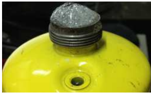
Valve Core Leak
