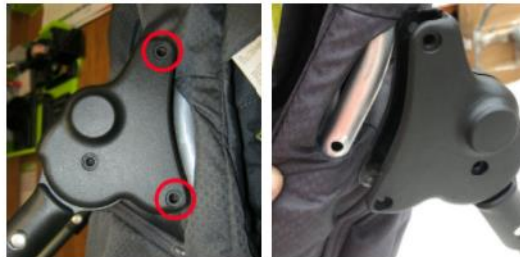
Bolt and washer missing
