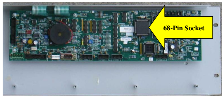
Figure 1 : Location of Microprocessor and 68-pin socket
