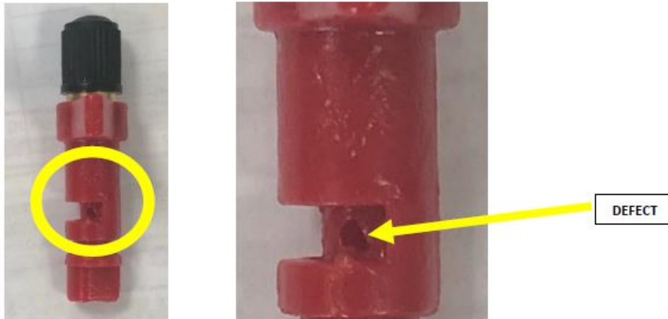
Figure 1: Photos of Service Valves showing defect
