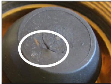
Separation of Rubber seal (Top)
