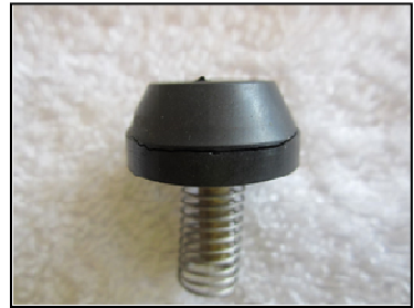
Separation of rubber seal (Side)
